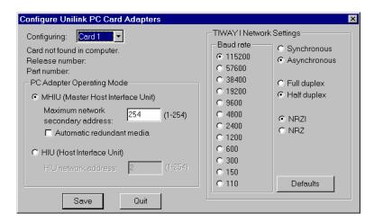
The settings in this dialog box are globally applied to all PLCs on the specified TIWAY network (each network requires a separate card). Therefore, it is only necessary to configure each Unilink PC Adapter one time—this step need not be repeated every time a new Tiway object is created.
