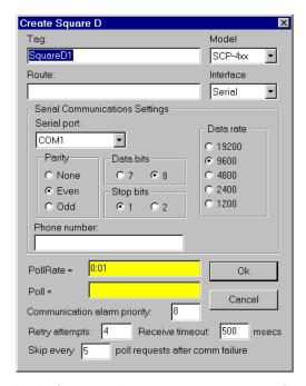
Figure 18-116. SquareD Definition Parameters Dialog Box Configured for Serial Communications
