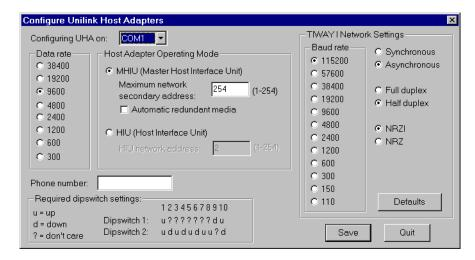
The settings in this dialog box are globally applied to all PLCs on the specified TIWAY network (each network requires a separate serial port). Therefore, it is only necessary to configure each Unilink Host Adapter one time— you need not repeat this step every time you create a new Tiway object.
