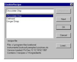
As you can see, the recipe names come from column A of the spreadsheet. You can use the *Previous* and **Next** buttons to identify a recipe from among the list, or type the name in the data entry field above the list. (This same dialog box appears later when an operator clicks on the pushbutton representing this object.) Click on **OK** to choose the recipe you want to use. Select the recipe for oatmeal cookies.
