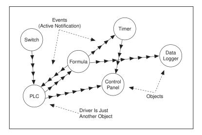
**Figure 2-5.** Lookout object-oriented and event-driven architecture
