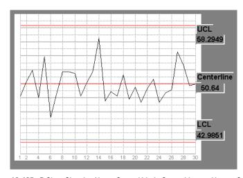
**Figure 18-135.** R Chart Showing Upper Control Limit, Center Line, and Lower Control Limits as Calculated Based on Plotted Samples.
