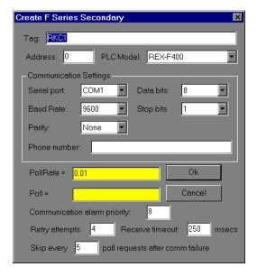
**Address** specifies which RKC F Series device you are communicating with. This number is between 0 and 31, and is set on the F Series device.
