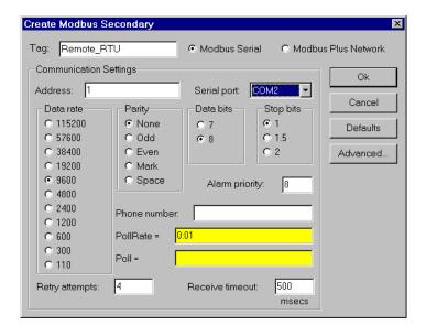
Because you are communicating through a remote radio to the RTU, you must select a serial port configured for radio communications. In this case, it's COM2.
