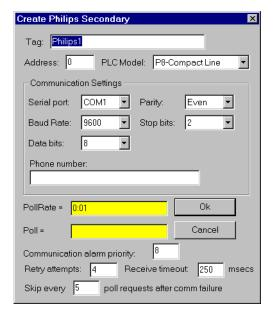
Figure 18-89. Philips Configuration Parameters Dialog Box
