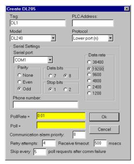
Figure 18-39. DL205 Parameters Configured for one PLC in a Multidropped Configuration
