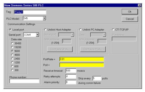
Figure 18-126. Tiway Configuration Parameters Dialog Box
