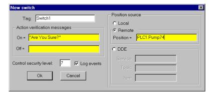
Figure 18-119. Switch Definition Parameters Dialog Box
