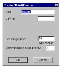
Figure 18-76. NIDAQ Device Configuration Parameters Dialog Box
