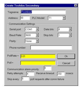
Figure 18-128. Toshiba T Series Configuration Parameters Dialog Box
