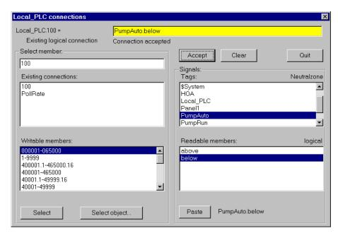
You now need to create another Modbus object for the remote RTU. Each controller has its own respective object in Lookout. Each of these objects determines its polling scheme, read/write blocking, and so on.
