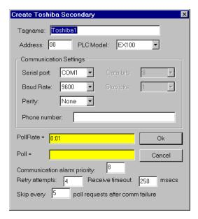
Figure 18-127. Toshiba M Series Configuration Parameters Dialog Box
