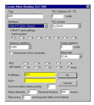
Figure 18-2. AB\_SLC-500 Definition Parameters Dialog Box Configured for DH+ Communications
