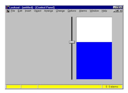
This bar graph simulates the water level in the tank. To give it a more realistic look, lay a graphic of a tank on top of it to act as a mask.
