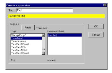
You can then connect this logical result to a PLC or RTU to control the fill valve. The valve opens when the tank level drops below 50 and closes when the tank level rises above 50. Notice, however, that this method can cause the valve to fluctuate between open and closed too often if the tank level hovers around 50.
