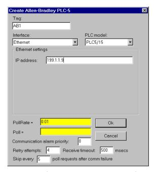
Figure 18-3. AB\_PLC5 Definition Parameters Dialog Box Configured for Ethernet Communications
