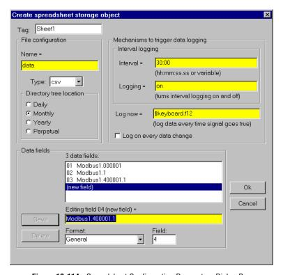
Figure 18-114. Spreadsheet Configuration Parameters Dialog Box
