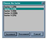
If you select the **Allow Decrement Count** option in the object definition dialog box, the Decrement button is displayed in the pop-up, allowing the operator to decrement a factor count. Operators with a high enough security level can correct errors if necessary.
