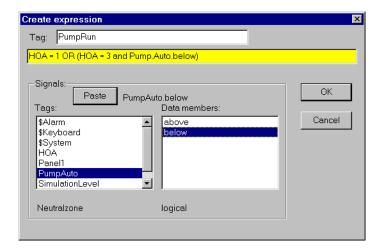
Notice the logic of the expression. If the HOA switch = 1 you are in the Hand position and want the pump to run, OR if the HOA switch = 3 you are in the Auto position AND you need to determine if the Neutralzone is calling for the pump to run (below specifies the signal is below the low limit and you need the pump to start). If the HOA switch = 2, you are in the Off position and the result of the expression is false.
