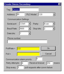
Figure 18-78. Omron Definition Parameters Dialog Box
