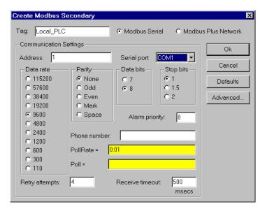
This is the local PLC located in the plant that controls the operation of the pump. Remember, you are hardwired to this PLC using COM1.
