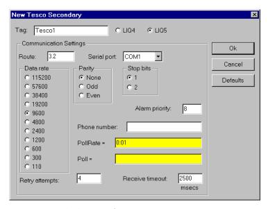
**Figure 18-121.** Tesco Configuration Parameters Dialog Box
